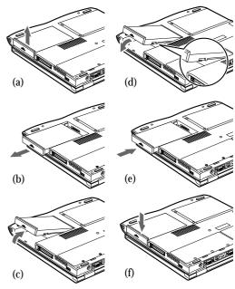
Figure 4-1 Replacing the Battery
